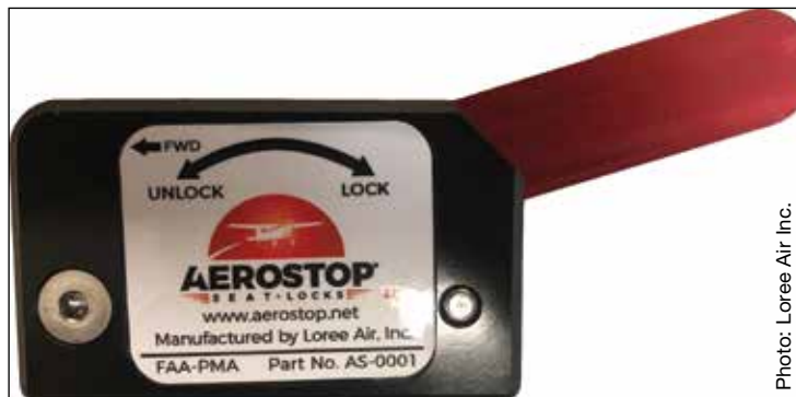
Loree Air offers the Aerostop seat lock secondary seat stop. This device slides over the Cessna seat rail and is secured using a lever, which applies a pressure pad on the top side of the seat rail.
