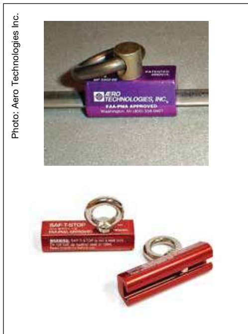
Aero Technologies' secondary seat stop, the Saf-T-Stop, is sold in pairs and slides over the pilot and copilot seat rails. Tightening the ring bolt puts pressure on the top of the seat rail. The company also makes a cargo ring for Cessna seat rails (topmost image).
